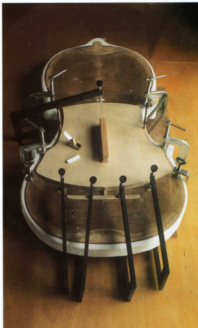
Figure 2. The back and mould set up in the traditional manner for patch fitting. A series of clamps around the edge of the patch area tries to prevent the back from springing up from the mould. This is quite ineffective at holding the back down in the centre of the patch area and only the rough preliminary fitting was done like this
