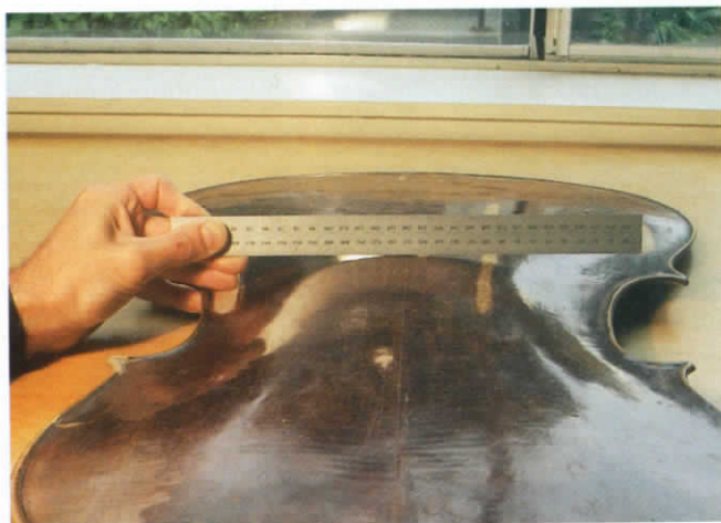
Figure 7b. The back arching after correction.
