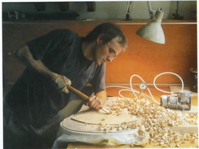
Figure 8. Trimming down the patch
