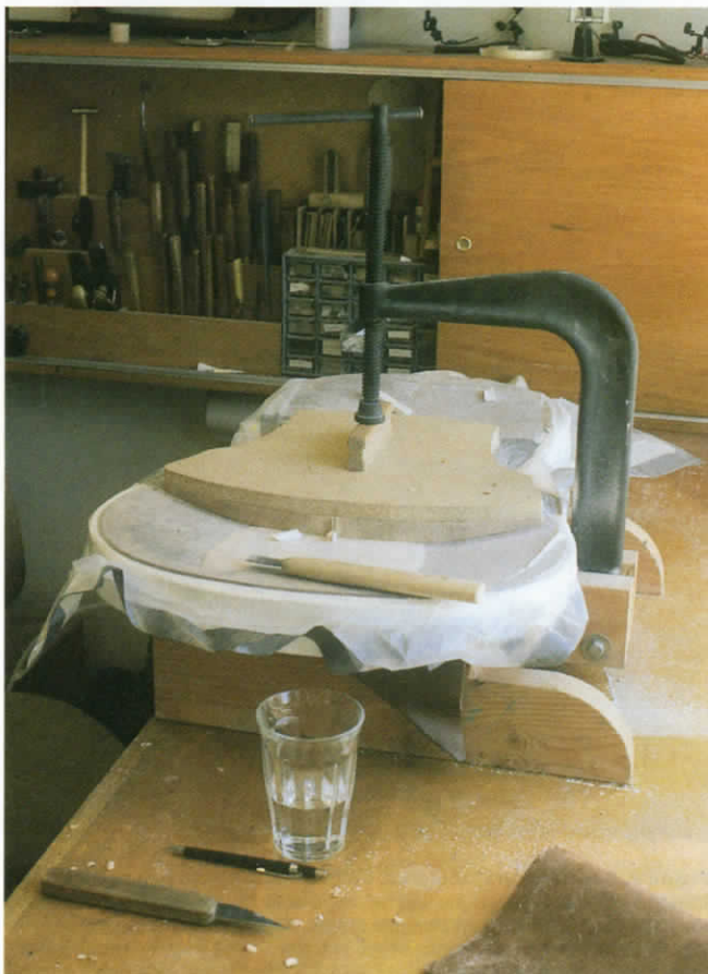
Figure 5. (left) The vacuum bag in use during chalk fitting. The vacuum holds the back firmly into the mould. The large c-clamp presses the patch into the back to take a chalk reading. A chipboard backer has been lightly glued to the patch to prevent the thin edges of the patch from flexing as the patch is clamped in place. The handle in the centre of the patch makes handling the patch easier during the hundreds of chalking and cutting operations
