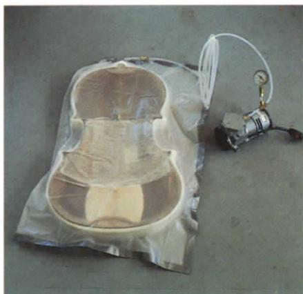
Figure 4. (below) A hole slightly larger than the patch is cut into the bag to allow access to the work area. The edges of the hole will be taped down to the cello back before the vacuum pump is turned on
