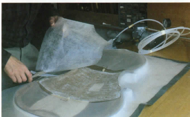
Figure 4. (below) A hole slightly larger than the patch is cut into the bag to allow access to the work area. The edges of the hole will be taped down to the cello back before the vacuum pump is turned on
